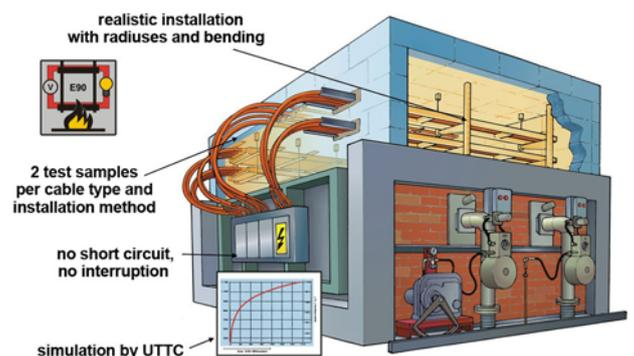
are obtained by directing the corresponding service through the test chamber several times.
