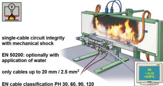
Figure 2: Testing a single cable in accordance with DIN VDE 0882-200 (previously: DIN VDE 0472-814), EN 50200, IEC 60331-25
