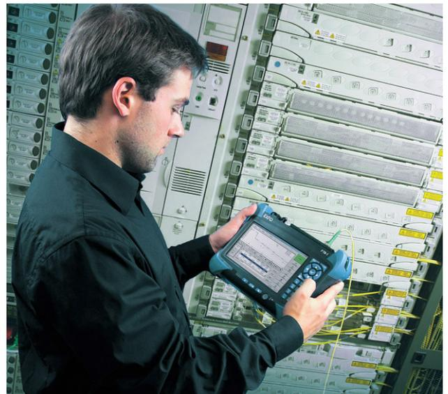
Image 1: OTDR testing a section of FO cabling. © EXFO/Opternus
