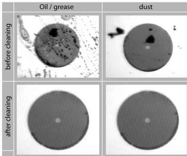
Image 4: Examples of contaminated and cleaned connector end faces.
